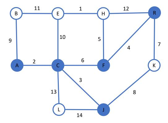
The graph above is a connected, unweighted graph where every edge has a unique weight between 1 and 12. We have been running Prim's Algorithm on this graph, beginning at node A. To this point, we have performed five iterations of the main loop, extracting five items from the priority queue. Those are the nodes filled in on the diagram above (i.e., nodes A, C, F, J, and R). Which is the next node extracted from the priority queue?
