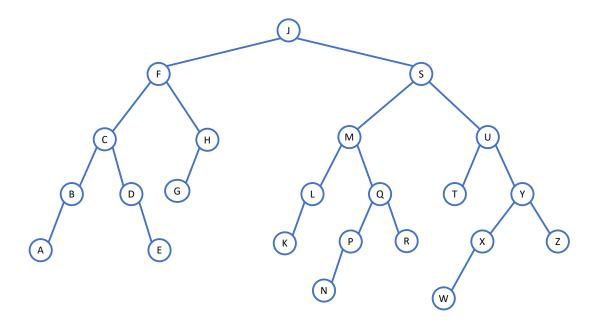
The tree above is an AVL tree, where some node has just been inserted, but no rebalance operations have yet been executed. The keys are letters of the alphabet, where A is smallest and Z is largest. Which node(s) are out of balance?
