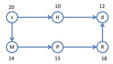
Here, the path from  $s \to H \to d$  has bottleneck speed 10, i.e., the slowest server on the path. On the other hand, the path from  $s \to M \to P \to R \to d$  has bottleneck speed 12.
