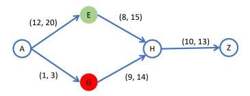
Here, node E is safe and node G is risky and the others are neutral. An edge with label (x,y) has safe cost x and risky cost y. There are two possible paths in this graph from A to Z: (i) via the safe node E at cost 30, or (ii) via the risky node G at cost 28. Thus in this case, the cheapeast path is  $A \to G \to H \to Z$ .
