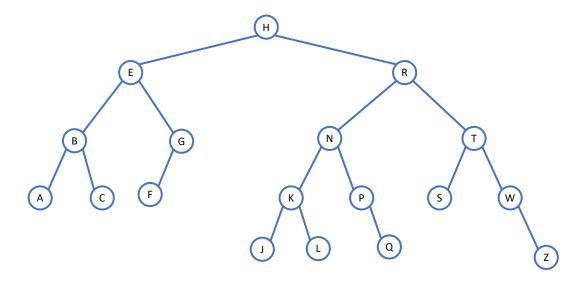
The tree above is an AVL tree. Assume that we insert M into the tree. Which rotation(s) occur? (Identify a rotation with the root of the subtree rotated. For example, a right-rotate(E) would move E down and B up.)
