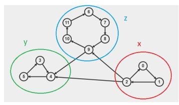
Suppose this is the original graph of dots and arrows. All vertices in SCC x (in red) are possible A', and all vertices in SCC y (in green) are possible B'. Vertices in SCC z (in blue) are neither possible A' nor B'.
