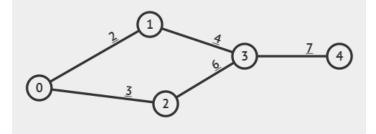
The best path from 0 to 4 will involve vertex 3, but instead of the path of least total expended energy from 0 to 3, which is 0-1-3 (total energy so far is 2), it should be using 0-2-3 (total energy so far is 3), since the path 0-1-3-4 uses 5 energy while 0-2-3-4 uses 4 energy only.
